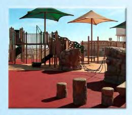
EnduraFlex is a more durable product, suitable for all age play areas, and may be installed indoors or outdoors. The materials are mixed and applied on-site so that the thickness can be modified to meet varying critical fall heights.
