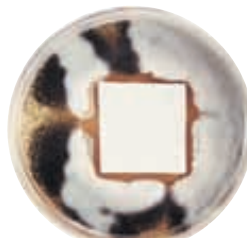
Mold growth is inhibited on the Foster® 40-20™ coating
