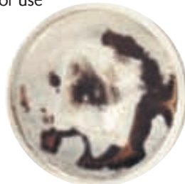
Mold covers the control sample completely.
