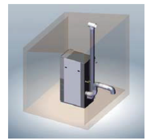
Vertical vent/sidewall air
