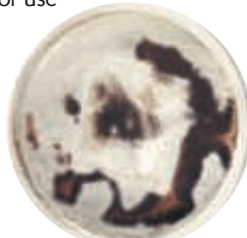
Mold covers the control sample completely
