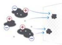
Airborne particles are charged by the ions causing them to cluster and be caught in filters
