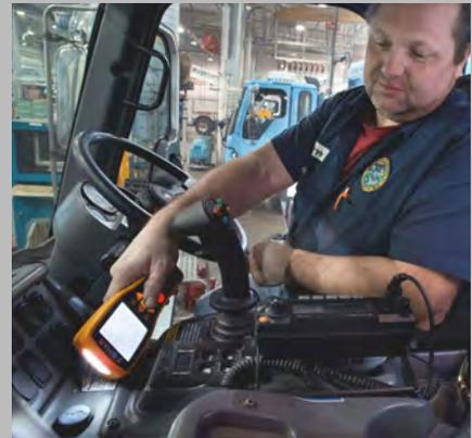
*Using Zonar’s 2010 inspection tool, the city’s drivers conduct their inspections by placing the reader within inches of each tag and indicating the condition of the components within the zone with one-handed, push-button responses.*
