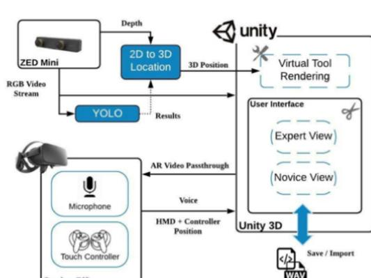
**Figure 5: (left) Hardware setup for implementation. The modified Oculus Rift VR head-mounted display supports video pass-through with a ZED mini depth camera to work in AR mode. Oculus touch controllers are tracked using external sensors. (right) System Architecture: The workspace is observed by the ZED mini depth camera, from which a 2D video feed is sent into Unity 3D to render an AR environment.**
