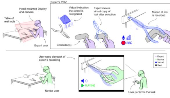
**Figure 6: First, Expert Users visually scan the set of tools available within their work space once. Upon recognition, virtual models of the tools and objects are rendered from the repository and can then be controlled with the aid of the controller. This enables the experts to record instructions along with voice instructions, which can then both be replayed for novice users later.**
