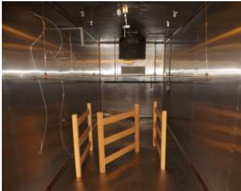
Figure 1 – Arrangement of the test bed headboards in the environmental chamber
